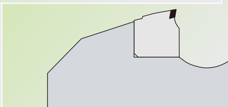
Tooth with positive hook angle for cutting solid
